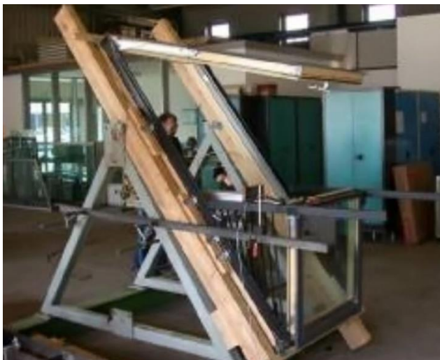
Figure 2.2.8.1 – Test rig with steel frame and section of wood rafter roof structure and the pressure pad
