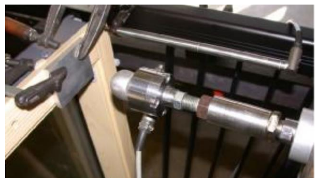
Figure 2.2.8.1 – Test rig with steel frame and section of wood rafter roof structure and the pressure pad
