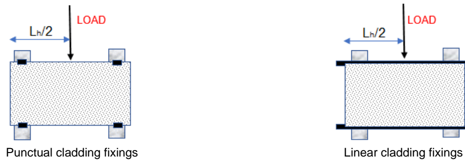
Figure J.1.1: Examples of test lay-out for punctual and linear cladding fixings when a subframe is used (cases a) and b) defined above). Frontal view,
