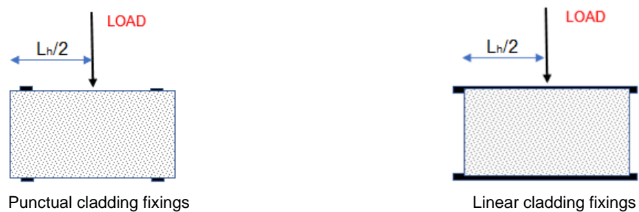
Figure J.1.2: Examples of test lay-out for punctual and linear cladding fixings installed directly to the substrate (case c) defined above). Frontal view,
