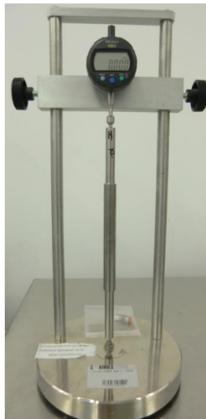
Figure D.2.1: Measuring device for dimensional variation, upper and lower contact elements ballpoint and standard bar
