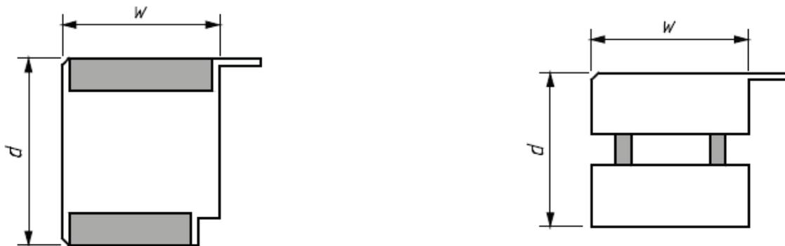
Figure A.23 – Width and depth of a profile
