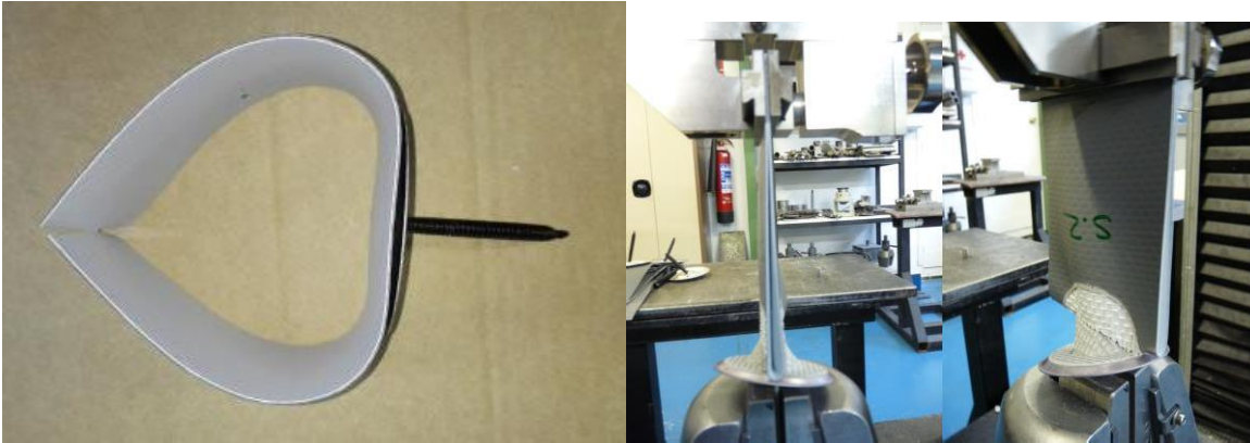
Picture 1. Peeling fastener-sheet
