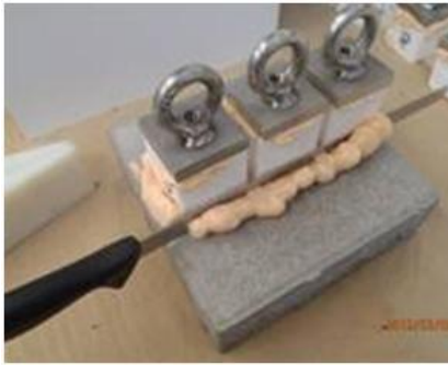
Figure C.2.7: Cutting of the surplus
