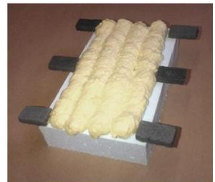
Figure C.2.3: Set-up with spacers (ex. 2)
