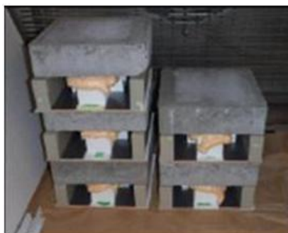
Figure C.2.5: Test sample during curing (48hrs)
