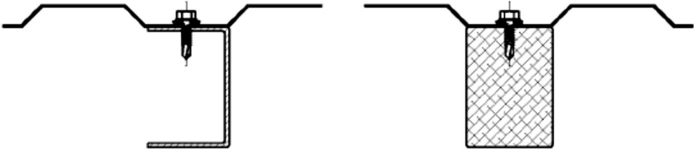
fastening of sheeting to a steel member
