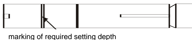
Figure 1.2 Fastener with internally threaded sleeve for in-place installation
